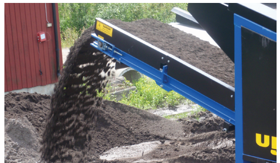
3 metre high material stockpile, on a 1.2 metre wide conveyor
